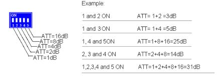
There are downlink (BTS site to )DIP Switches (Hi ATT) and uplink DIP Switches (Lo ATT) for single band.
